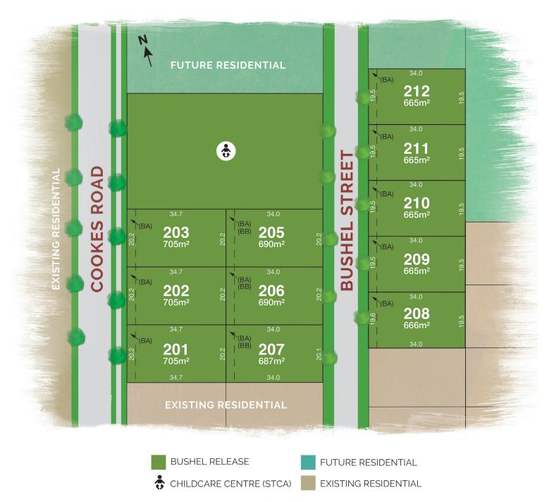
(BA) EASEMENT FOR DRAINAGE OF SEWAGE 3 WIDE (BB) EASEMENT FOR DRAINAGE OF WATER 3 WIDE ALL DIMENSIONS AND AREAS ARE SUBJECT TO FINAL SURVEY.
