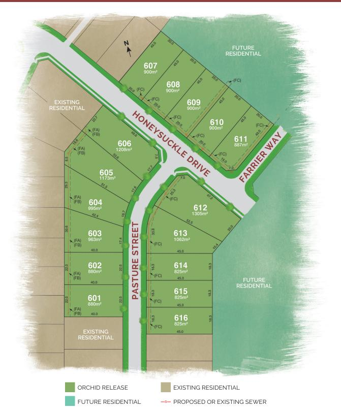
(FA) EASEMENT FOR DRAINAGE OF SEWAGE 4 WIDE (FB) EASEMENT FOR DRAINAGE OF WATER 4 WIDE (FC) EASEMENT FOR DRAINAGE OF SEWAGE 3 WIDE
