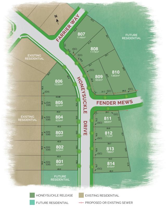
(GA) EASEMENT FOR DRAINAGE OF SEWAGE 4 WIDE (GB) EASEMENT FOR DRAINAGE OF WATER 4 WIDE (GC) EASEMENT FOR DRAINAGE OF SEWAGE 3 WIDE
